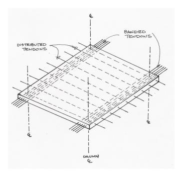
Figure 4: Typical post-tensioning tendon layout.
