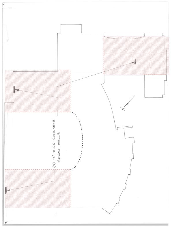
Figure 8: Location of the three shear walls designed to resist the lateral loads. Red hatch shows area of influence.
