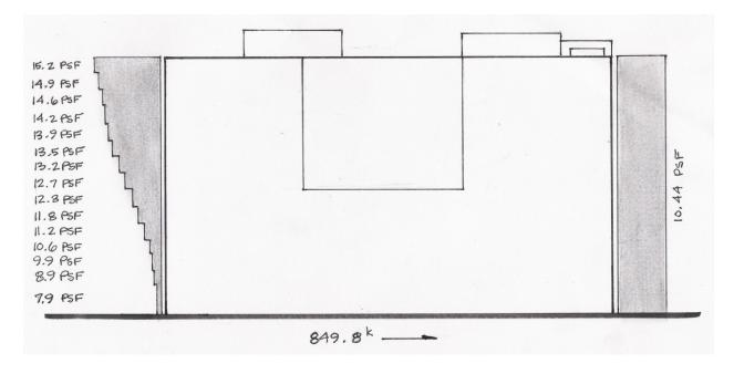
Wind Loading Diagram for East - West Direction:
