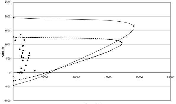
Interaction Diagram for Frame 6 using 1.2D + 1.0L + 1.6W
