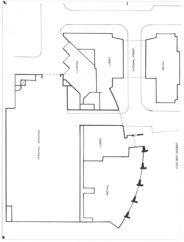
Figure 6: First Floor and Overall Site Plan showing overall shape for lower floors.
